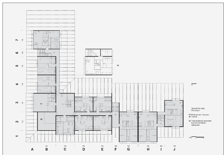
FIG. 2 SECOND-FLOOR PLAN OF THE FIRST PHASE OF THE “DEPARTMENT STORE” MIXED-USE BUILDING, PRESENTED TOGETHER WITH A THREE-BEDROOM APARTMENT FROM THE THIRD FLOOR. SECOND FLOOR INCLUDES A KINDERGARTEN – DAYCARE, A LARGE CORNER TERRACE, AND ELEVEN RESIDENTIAL UNITS, 1973
