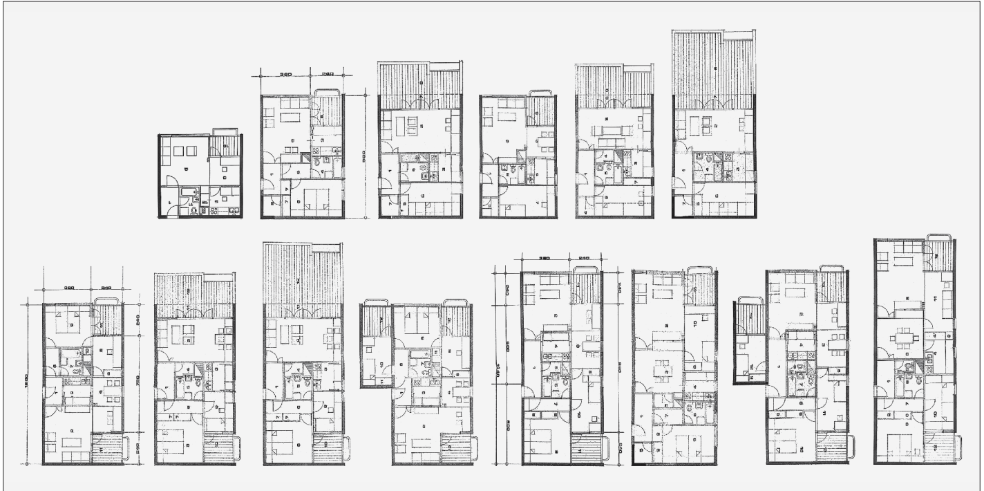
FIG. 9 TYPOLOGY OF THE APARTMENTS IN ELONGATED BUILDING D2, RANGING FROM STUDIO TO THREE BEDROOM APARTMENTS. APARTMENTS FEATURE FLEXIBLE LAYOUT DUE TO FIXED CENTRAL CORE AND REMOVABLE PARTITIONS. MOST UNITS ARE CONCEIVED WITH CIRCULAR CONNECTION
