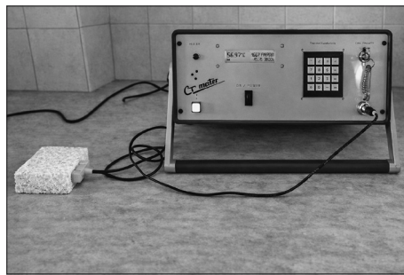
FIG. 6 EXPERIMENTAL SETUP FOR MEASURING THERMAL CONDUCTIVITY AND SPECIFIC HEAT (TC-METER). (SOURCE: AUTHORS, 2022)
