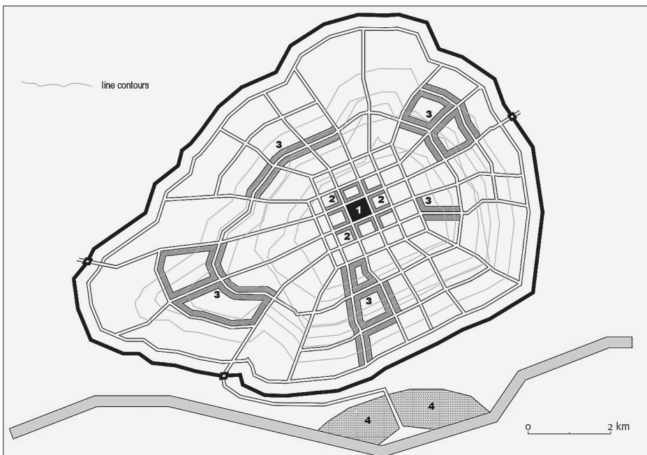
FIG. 3 FICTIONAL MEDIEVAL CITY LAY-OUT SCHEME, 1 MARKET ZONES, 2 CRAFT ZONES, 3 CRAFT AND TRADE ZONES (E.G. SHOEMAKERS' STREET, BLACKSMITHS' STREET), 4 LARGE MANUFACTURING WORKSHOP ZONES
