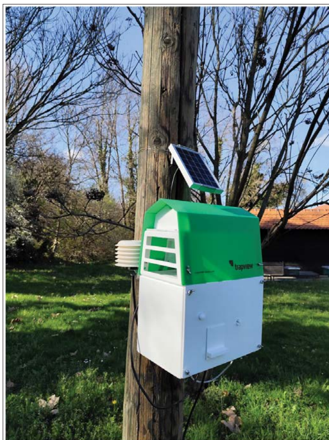
Figure 7. Camera-based smart trap used for automated insect monitoring and data collection under field conditions (Helena Viric Gasparic, Zagreb, Croatia)
