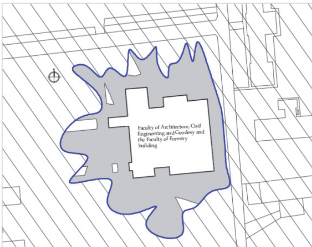
Figure 3 Admissible area (non-hatched regions outside the object) for scanner placement for scanning the building of the Faculty of Architecture, Civil Engineering and Geodesy and the Faculty of Forestry at an incidence angle of \alpha_{\max} = 65^\circ . The blue line represents the maximum allowable scanner distance, determined based on obstacles present in the field
