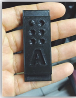
Figure 7 Key designed for the keyboard and printed with the Creality Ender V2 3D printer
