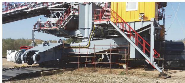
Figure 3 Drive wheel and caterpillar shoe chain connected by cylindrical links
