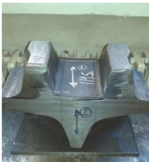
Figure 11 Appearance of the delivered part of the shoe link with marked sampling directions
