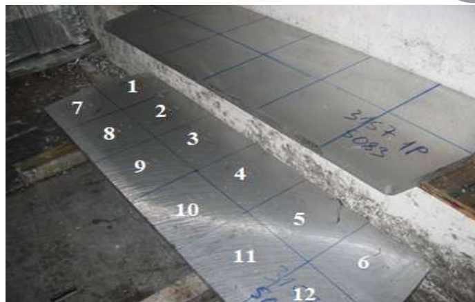
Figure 1. Cross-sections of plates cut from the front and rear sections of the EN AW-5083 alloy ingot (charge 3157), showing the sampling layout consisting of twelve segments (positions 1–12).
