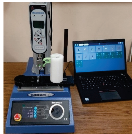
Figure 13 MultiTest-dV testing machine
