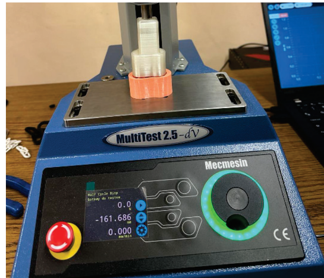
Figure 7. Position the sample on the platform under the punch before the compression test
