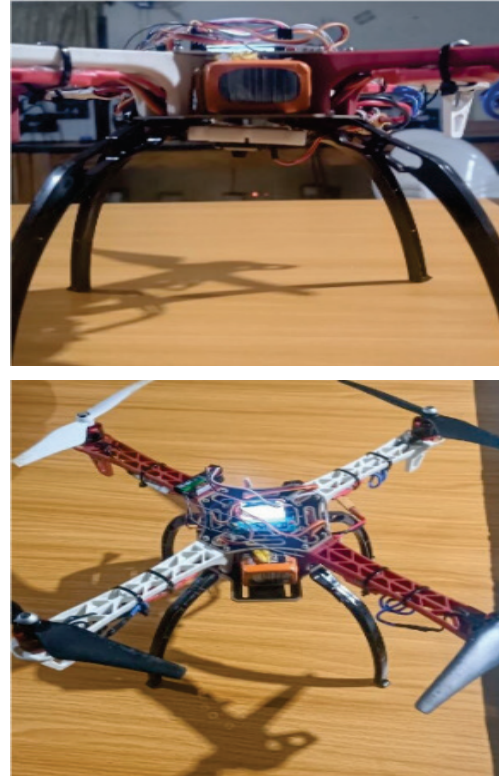
Figure 9 Custom-designed drone with mounted Raspberry Pi 5 and camera module
