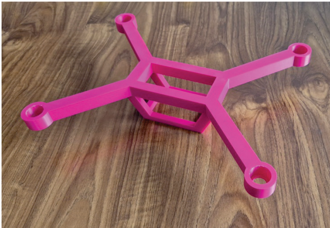
Figure 4 A prototype of a drone structure made on the basis of a 3D-CAD model using the 3D printing method
