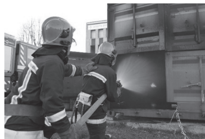
Figure 15. Supplying the fine spray from the Protek 366 nozzle inside the CFS
