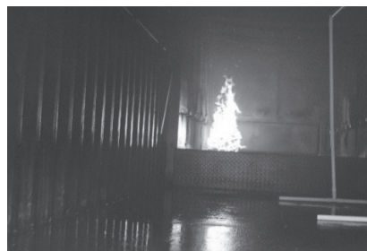
Figure 7. A fire of a stack of wooden boards in the container
