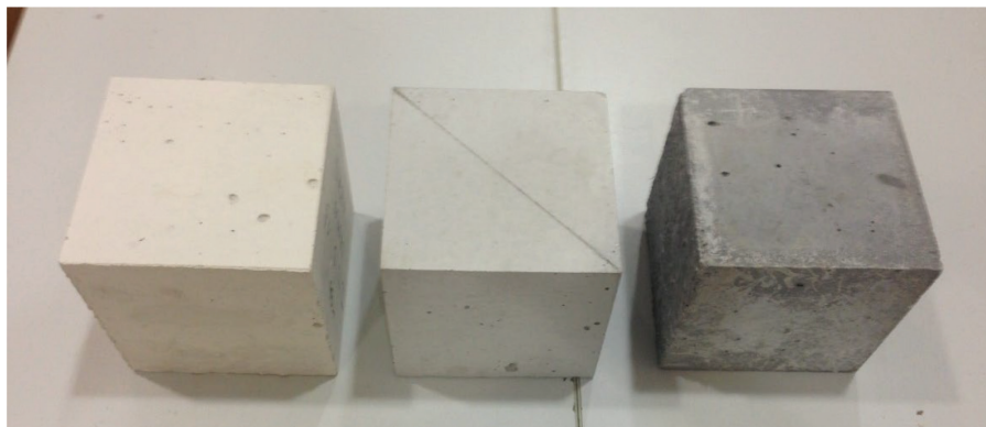
Fig. 5: Comparison of whiteness of samples produced using white cement (left), GC with titanium dioxide and metakaolin (centre) and GC (right). GC, grey cement.
