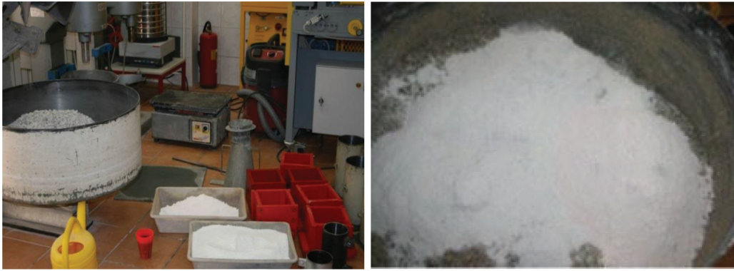
Fig. 3: Laboratory mixer, concrete components, vibrating table (left), white cement and metakaolin (right).
