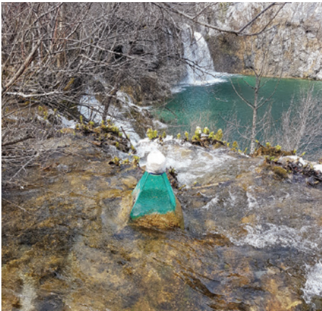
Fig. 3. Pyramid-shaped emergence trap at the Kozjak-Milanovac tufa barrier. Photo by: M. Ivković
