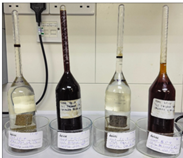
Figure 5: Spontaneous Imbibition Using Amott Cell
