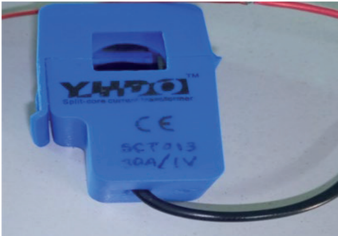
Fig. 4. SCT-013 Current Transformer
