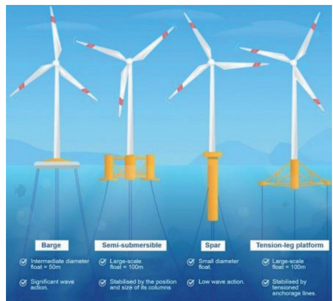
Fig. 6. Types of foundations for floating wind farms
