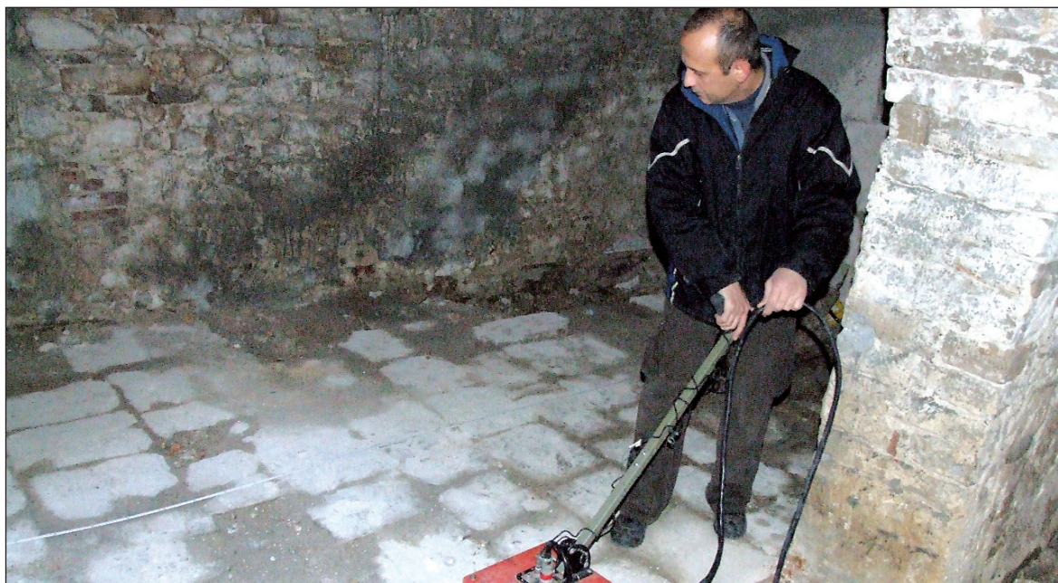
Sl. 13. Istraživanje u podrumu kuće Andrić u Splitu s antenom od 400 MHz Fig. 13. Investigation in the cellar of the Andrić house in Split with a 400 MHz antenna
