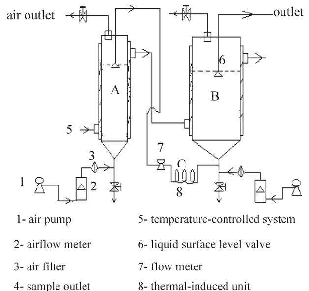
Fig. 1 – Diagram of three-stage process system for continuous fermentation of PGA
