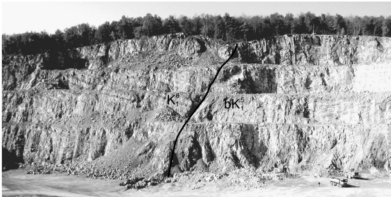
Fig. 8 Tounj quarry. Fault contact (in the centre of the photograph) of well-bedded Albian limestones ( K_1^6 , on the left) and thick-bedded to massive Lower Aptian rudist limestones ( bk_1^5 , on the right). Elevation from the bottom to the top of the quarry is approx. 80 m, comprising an approximately equally thick part of the Lower Aptian succession.
