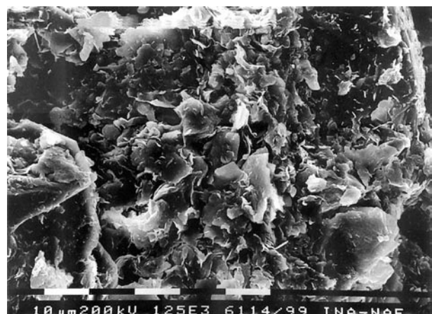
Fig. 14 SEM photomicrograph of the gray-coloured silty clay. Clusters of fine flaky chlorite surrounded by quartz particles are quite frequent.
