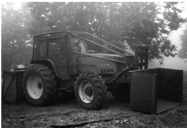
Fig. 2 Valtra Valmet 6050 tractor (75 kW) forestry version, equipped with open-ended containers mounted on both front and rear sides
