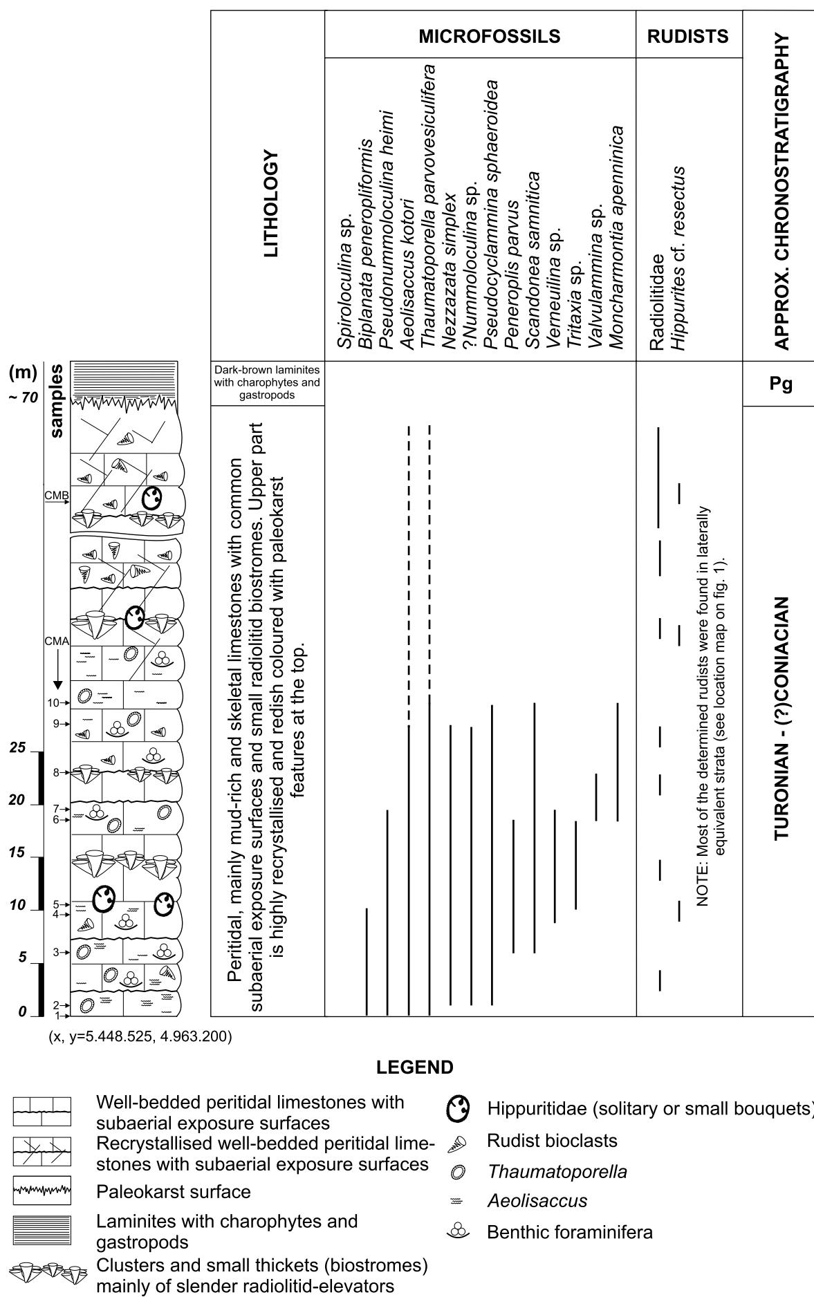
Fig. 2 Stratigraphic distribution of microfossils and rudists within the Martinšćica section (modified after KORBAR, 1999).
