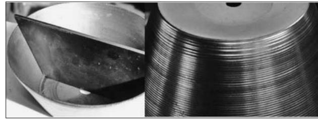
Figure 8a, b. Checking the insert height, draw piece with furrows on the surface
