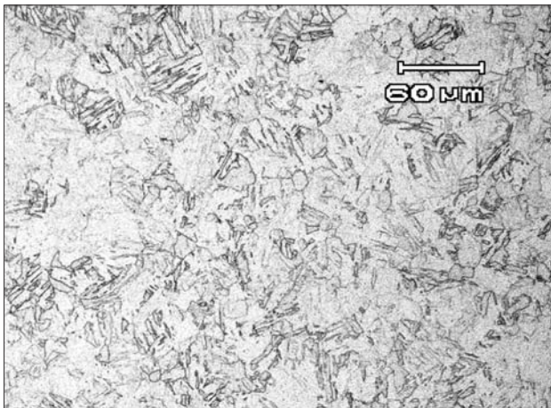
Figure 1. Microstructure of quenched steel X2CrNiMo 13-6-2
