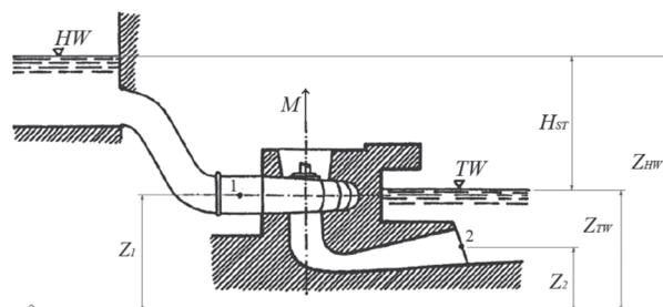
**Figure 1.** Measurement point schematic for Francis turbine hydraulic characteristics
