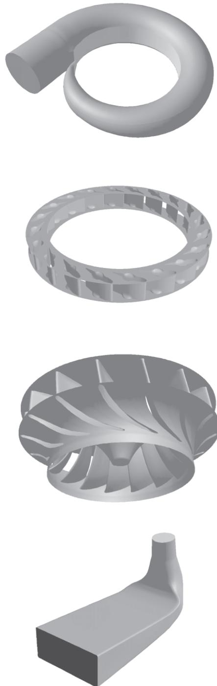
**Figure 3.** Partitions of the turbine geometry
