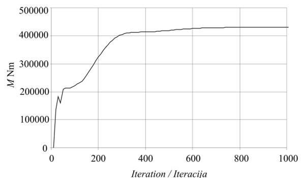
**Figure 7.** Convergence history for the turbine runner torque
