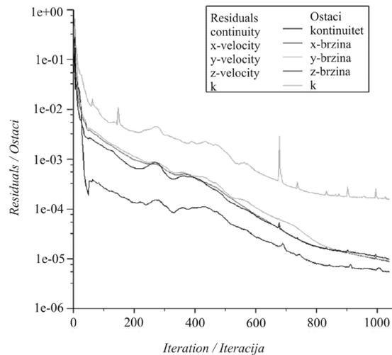
**Figure 5.** Residuals (a measure of discretized equation solution inaccuracy)
