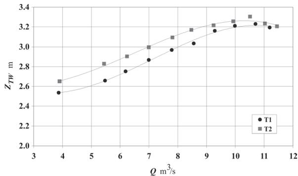
**Figure 2.** Tailwater level for individual operation of turbines T1 and T2
