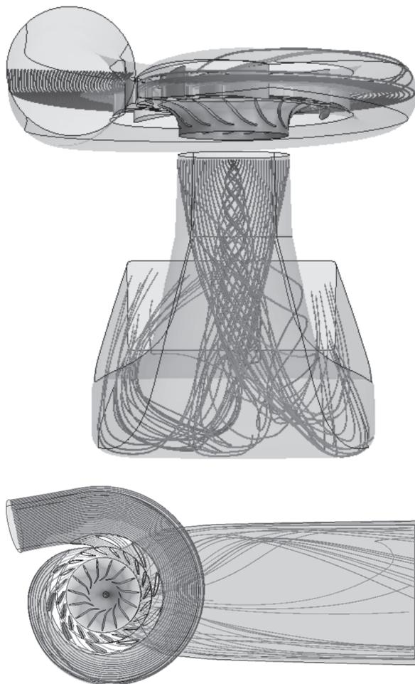
Figure 12. Fluid flow pathlines in the HPP Rijeka turbine, colored by total pressure, 100 % HKSM
