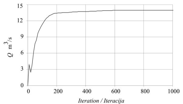
**Figure 6.** Convergence history for the inlet section volumetric flow rate
