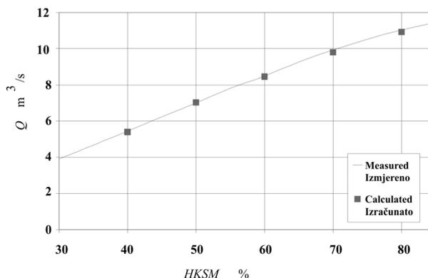
**Figure 9.** Comparison of computed and measured volumetric flow rate over HKSM; single mode T2
