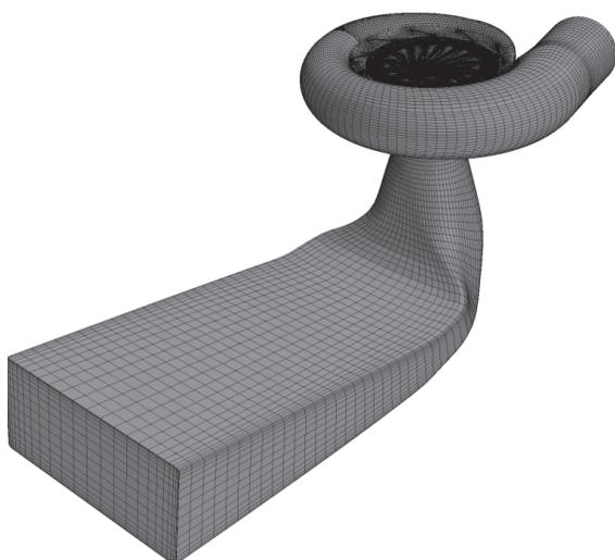
**Figure 4.** Numerical mesh surface of control volumes for the HPP Rijeka turbine
