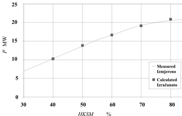
**Figure 8.** Comparison of computed and measured power over HKSM; single mode T2
