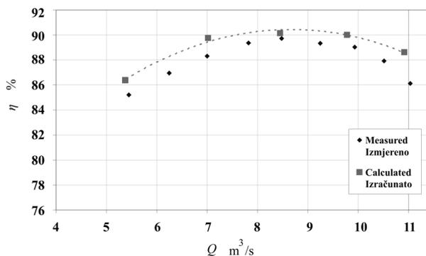
**Figure 10.** Comparison of computed and measured turbine efficiency over volumetric flow rate; single mode T2
