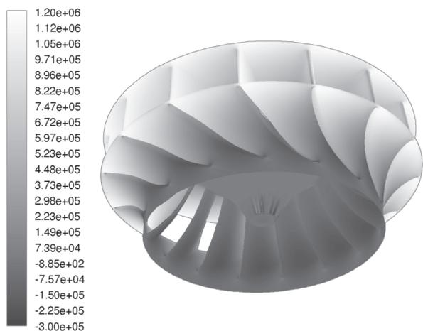
Figure 11. Contours of static pressure on runner surfaces
