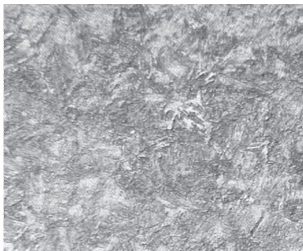
**Figure 10.** Microstructure of the substrate under the coating, 250x magnification, etching: nital solution
