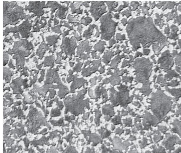
**Figure 6.** Microstructure of the substrate under the coating, 250x magnification, etching: nital solution
