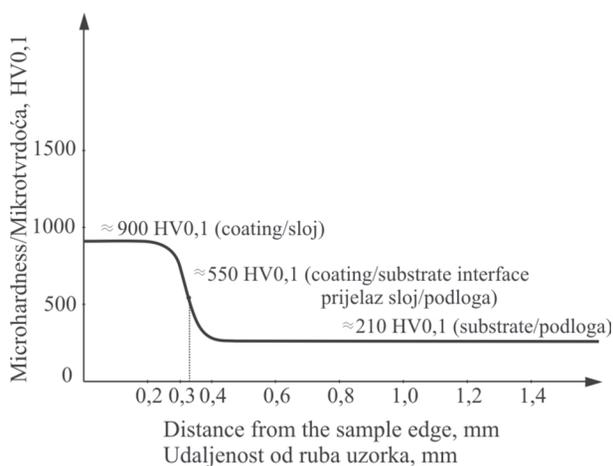
**Figure 8.** The results of microhardness measurements for the sample NiCrBSi coating-C45 steel
