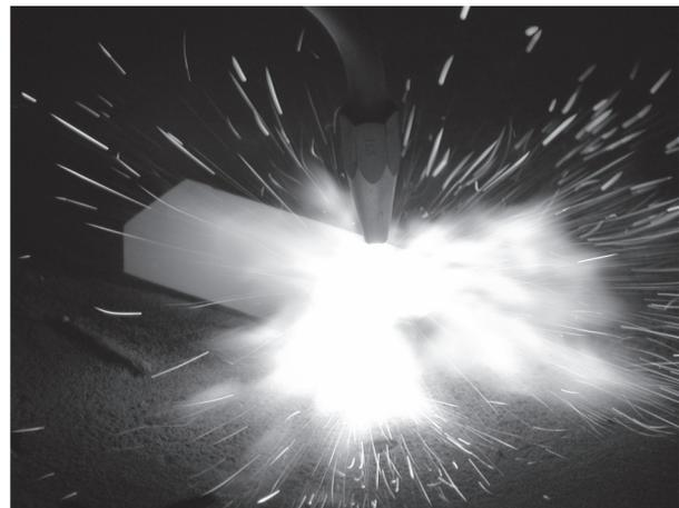
**Figure 1.** Flame spraying and simultaneous fusing
