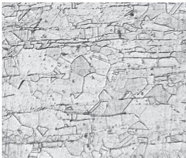
**Figure 15.** Microstructure of the substrate remote from the coating, 250x magnification, etching: glyceresia
