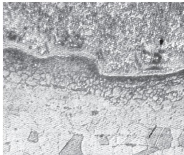
**Figure 13.** Microstructure of the cross sectioned sample: NiCrWBSi coating-X6CrNiMo18-10-2 steel substrate, 450x magnification, etching: glyceresia
