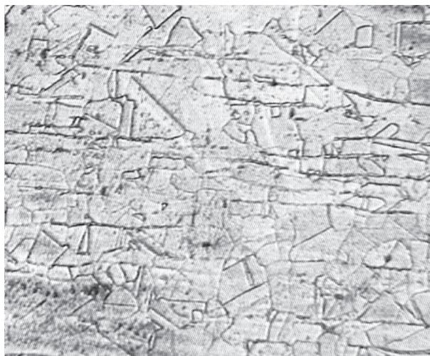
**Figure 14.** Microstructure of the substrate under the coating, 250x magnification, etching: glyceresia
