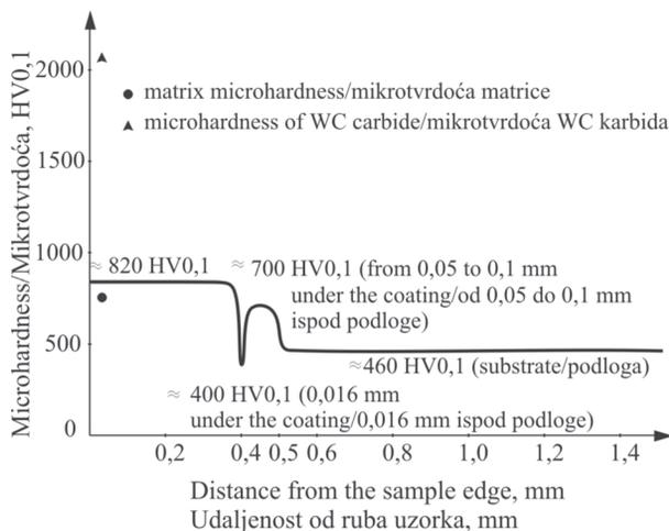
**Figure 12.** The results of microhardness measurements for the sample NiCrBSi+WC coating-42CrMo4 steel
