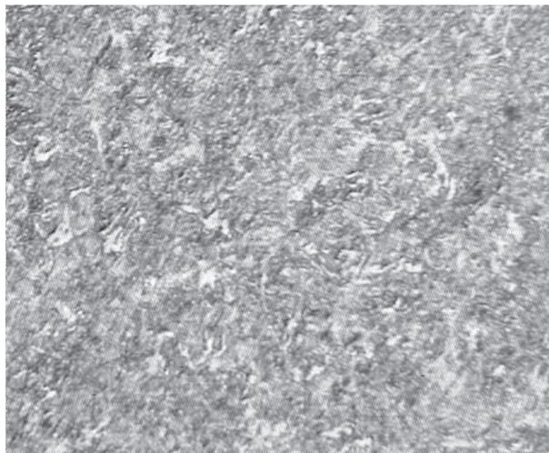
**Figure 11.** Microstructure of the substrate remote from the coating, 250x magnification, etching: nital solution
