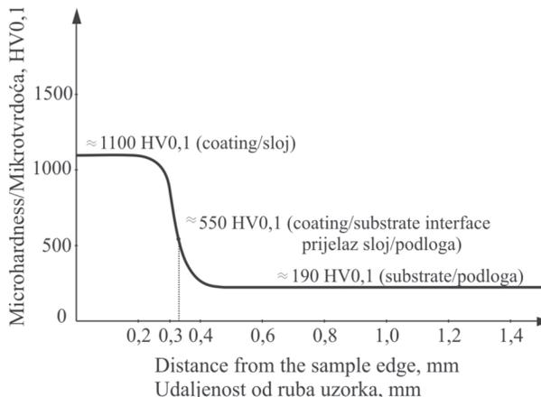
**Figure 16.** The results of microhardness measurements for the sample NiCrWBSi coating- X6CrNiMo18-10-2 steel
