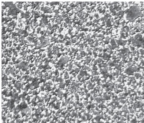
**Figure 7.** Microstructure of the substrate remote from the coating, 250x magnification, etching: nital solution
