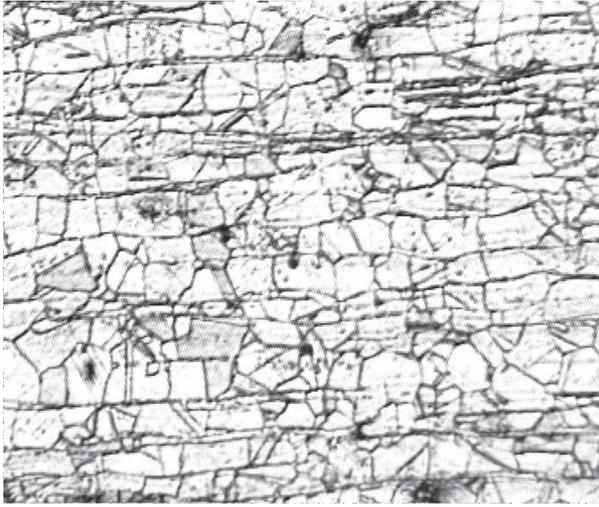
**Figure 4.** Microstructure of stainless steel X6CrNiMo18-10-2 (cross section of the sample, 250x magnification, etching: glyceresia)
