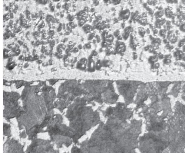
**Figure 5.** Microstructure of the cross sectioned sample: NiCrBSi coating-C45 steel substrate, 450x magnification, etching: nital solution
