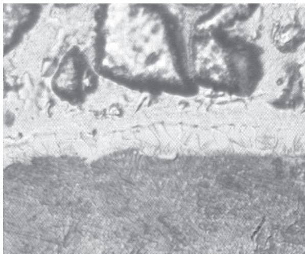
**Figure 9.** Microstructure of the cross sectioned sample: NiCrBSi+WC coating-42CrMo4 steel substrate, 450x magnification, etching: nital solution
