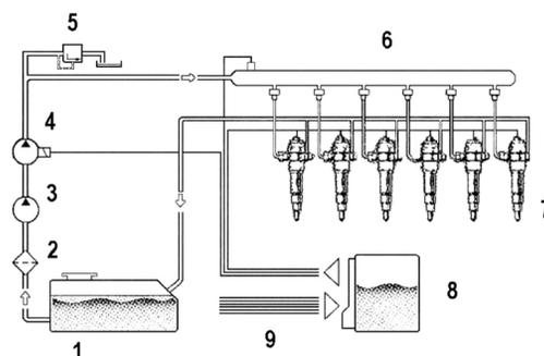
**Figure 1.** Common rail fuel system:
