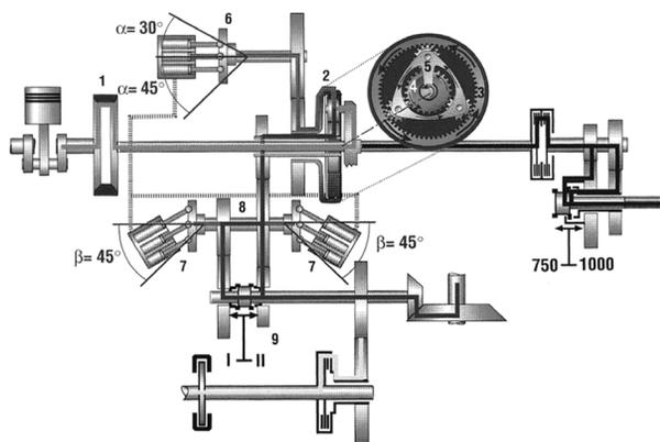
**Figure 4.** Continuously variable transmission (CVT):
