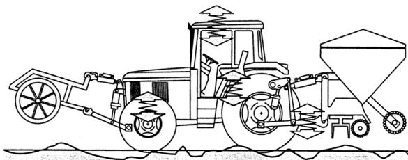
**Figure 7.** Vibration damping system
