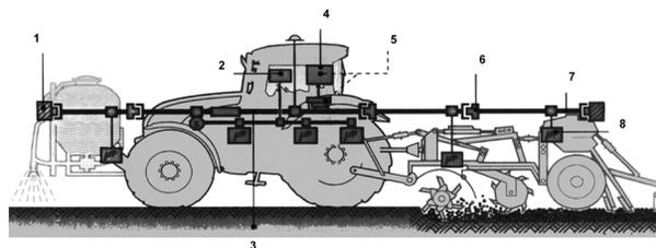
**Figure 9.** Communication between tractor and implement using ISO Bus: 1. Bus terminator, 2. Tractor internal monitor, 3. Tractor internal Bus, 4. Bus terminal, 5. Data transfer to management computer, 6. Bus connector, 7. Tractor implement Bus, 8. Electronic control unit (ECU)
