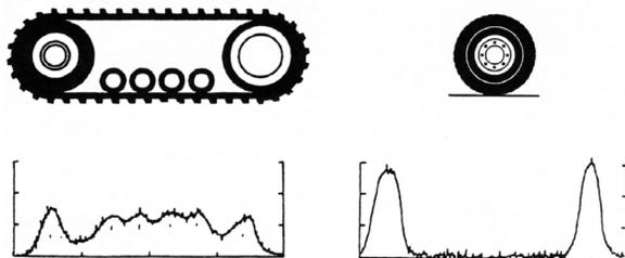
**Figure 11.** Contact pressure at tractor with rubber belt and wheels
