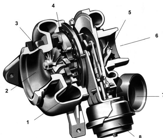
**Figure 3.** Variable geometry turbocharger (VGT): 1. Exhaust-inlet, 2. Exhaust-outlet, 3. Turbine wheel, 4. Moveble vanes, 5. Charger wheel, 6. Air intlet 7. Air-outlet, 8. Membrane actuator
