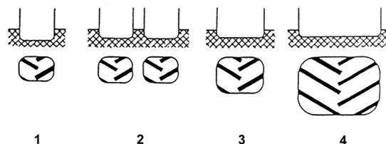
**Figure 10.** Contact area of different tractor tires: 1. Standard, 2. Dual, 3. Wide, 4. Terra
