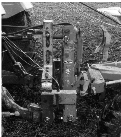
Figure 4. Attaching of dynamometer frame and direction of measured forces
