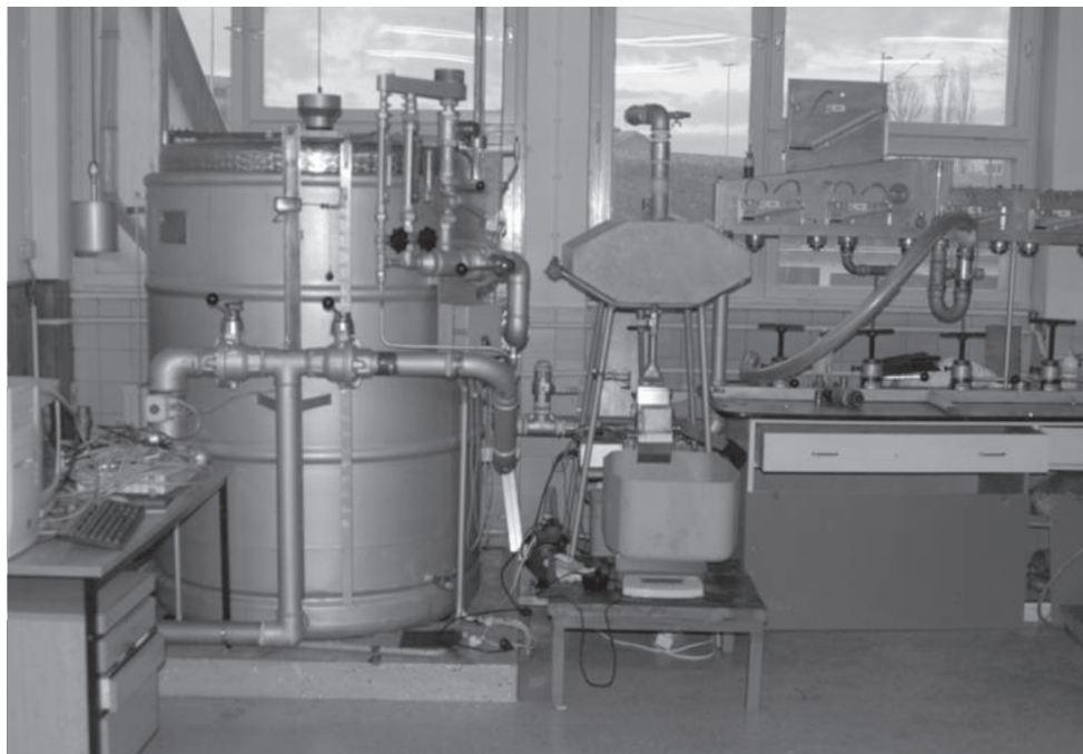
Figure 1. System for calibrating gas flow standards in the Zagreb Gasworks
