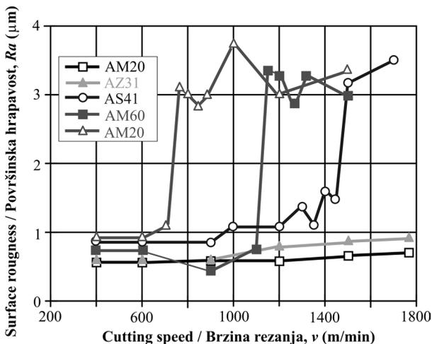
Figure 2. The variation of surface roughness (Ra) versus cutting speed (v) for five magnesium alloys
