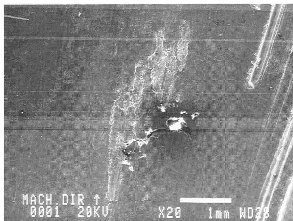
**Figure 6.** Porosity found in magnesium alloy AZ91
