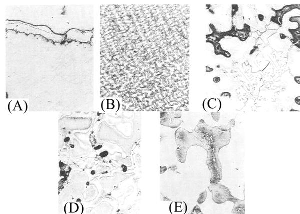
**Figure 1.** Typical microstructures of A) AM 20, B) AZ 31, C) AS 41, D) AM 60 and E) AZ 91
