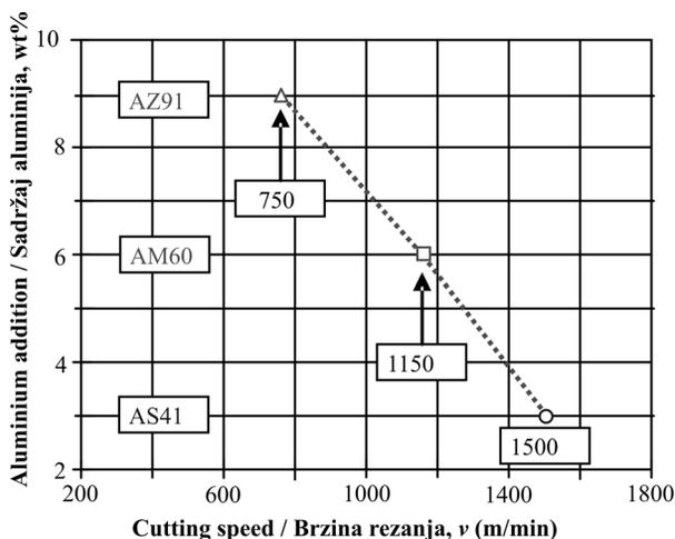
Figure 3. Effect of aluminium content on critical cutting speed (formation of FBU)
