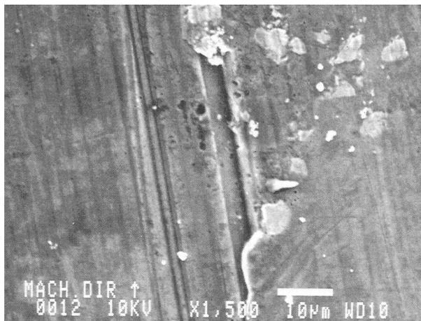
**Figure 4.** Damage of the machined surface caused by MnAl hard particles which have been moved by the cutting edge and thus made grooves
