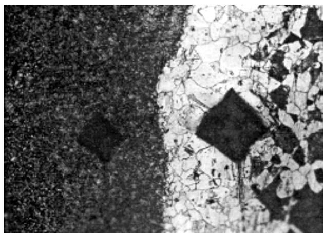
Figure 7 Microstructure in the area of joining (200×)
