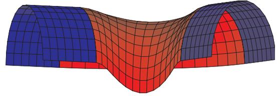
Figure 4:  $G^1$  continuous input data result  $G^1$  connection.
