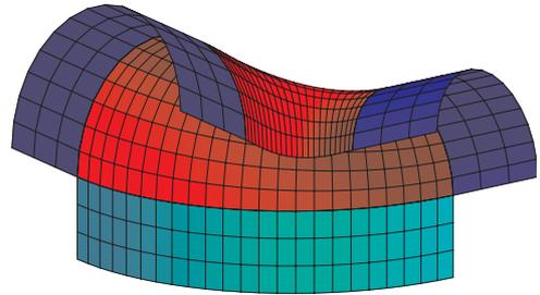
Figure 6: Combination of three surfaces,  $G^1$  connection
