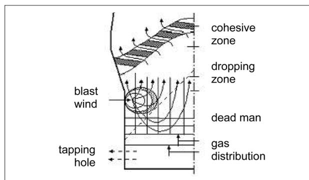
Figure 1. Lower parts of the blast furnace
