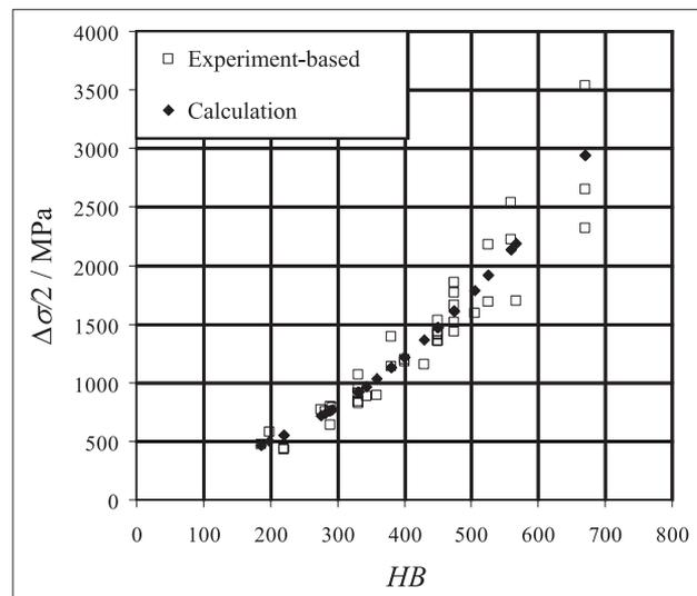
Figure 5. Values of  $\Delta\sigma/2$  calculated for  $\Delta\varepsilon_p/2 = 2\%$
