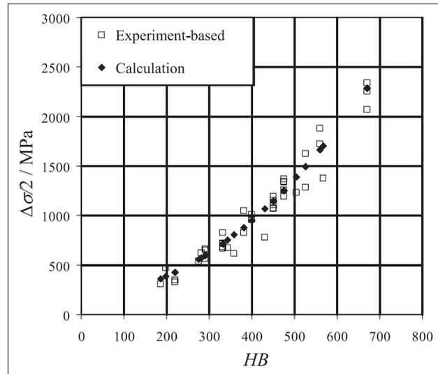
Figure 4. Values of  $\Delta\sigma/2$  calculated for  $\Delta\varepsilon_p/2 = 0,2\%$
