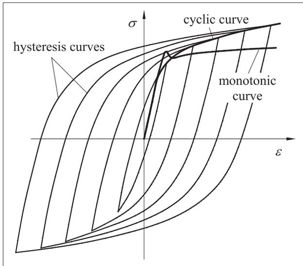
Figure 1. Stress-strain curves
