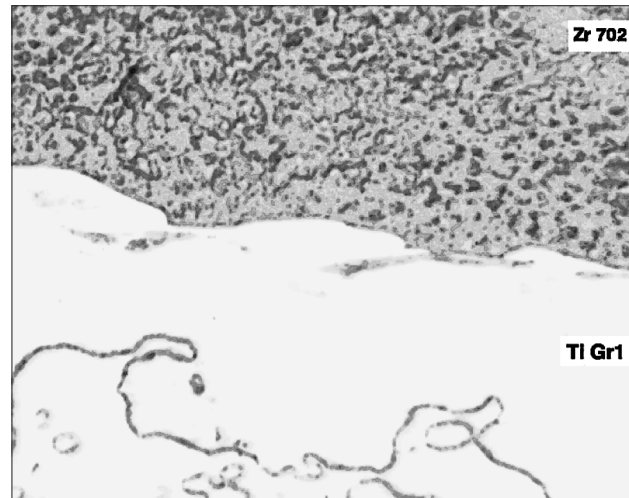
Figure 4. Transition area Ti/Zr. Magnif. 100 ×
