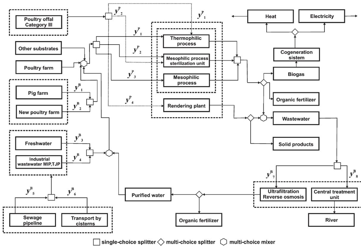
Fig. 2 – Superstructure for selecting the optimal processing system for the industrial case study
