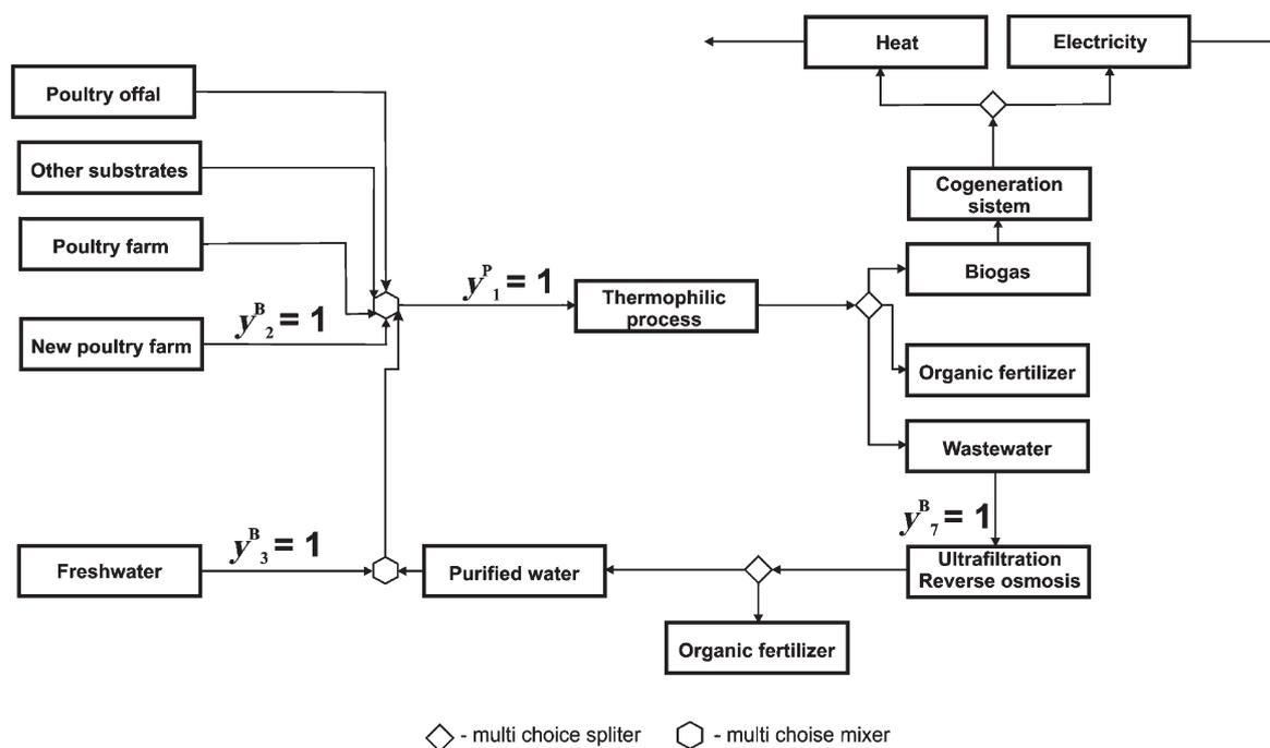
Fig. 3 – Optimal solution for the industrial case study of biogas production in a thermophilic process without a rendering plant
