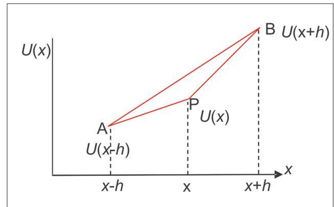
Fig. 1. Geometrical representation of finite difference method
