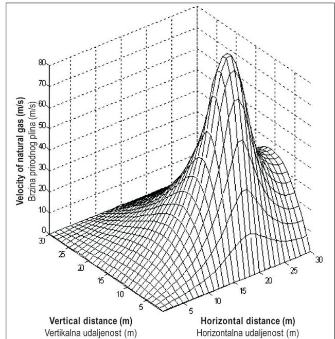
**Fig. 3. Velocity profile in the horizontal and vertical directions for the gas from rupture point**
