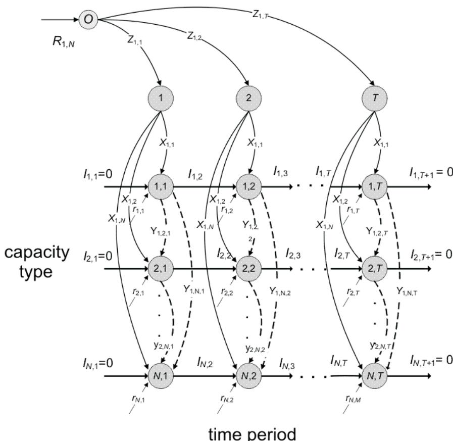
Figure 2 A network flow representation of the capacity expansion problem
