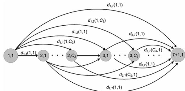
Figure 3 The CEP problem can be seen as the shortest path problem for an acyclic network of calculated CESs
