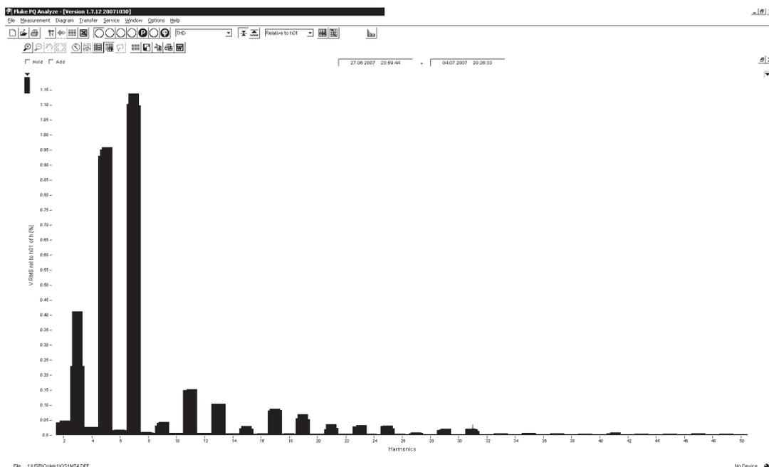
**Figure 15** Harmonic spectrum of 10 kV voltage level at MT4
