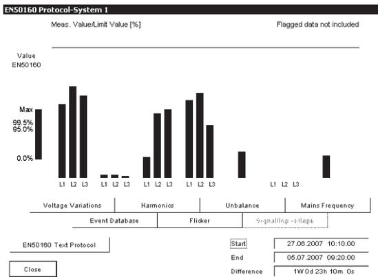
Figure 10 Summary power quality indices at 110 kV voltage level at MT1
