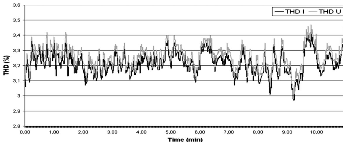
Figure 4 Period diagram THDU and THDI for pure linear load
