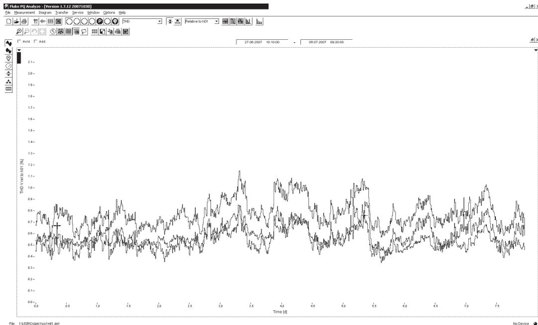
Figure 12 Total voltage harmonic distortions  $THD_v$  at 110 kV level at MT1
