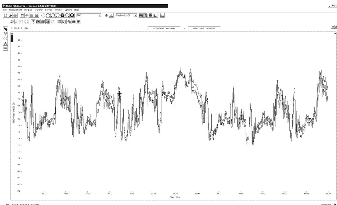
**Figure 14** Total voltage harmonic distortions  $THD_v$  at 0,4 kV level at MT6
