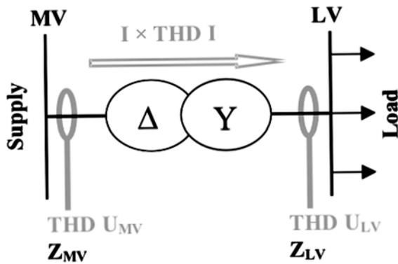
Figure 7 Simultaneous measurement on MV and LV side
