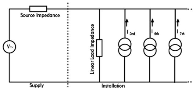
Figure 3 Equivalent non-linear load circuit
