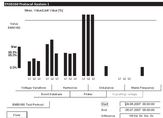
Figure 11 Summary power quality indices at 10 kV voltage level at MT4
