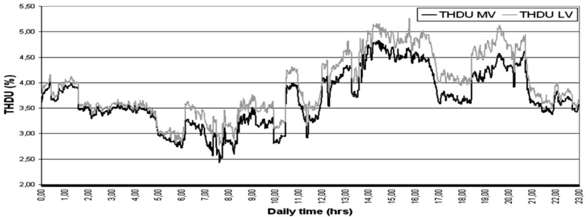
Figure 8 Simultaneous period diagram recorded  $THDU_{MV}$  and  $THDU_{LV}$
