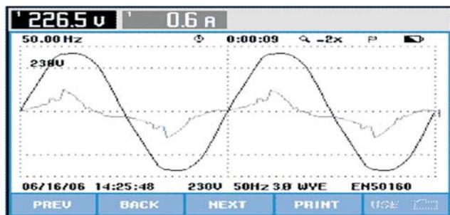
Figure 1 Current and voltage waveform
