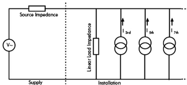
Figure 3 Equivalent non-linear load circuit
