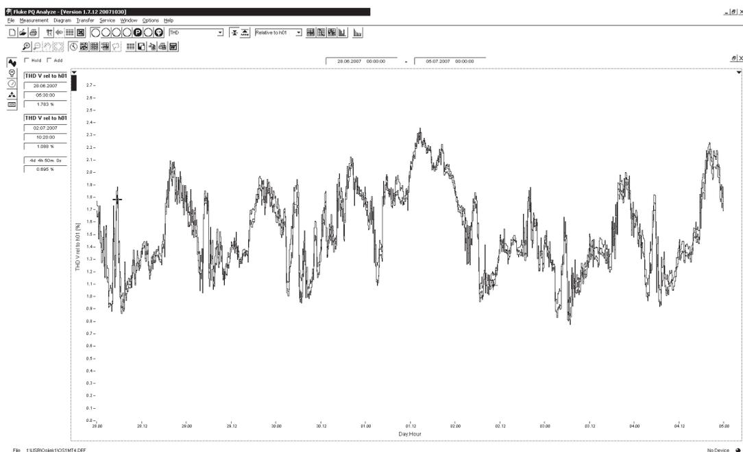
**Figure 13** Total voltage harmonic distortions  $THD_v$  at 10 kV level at MT4
