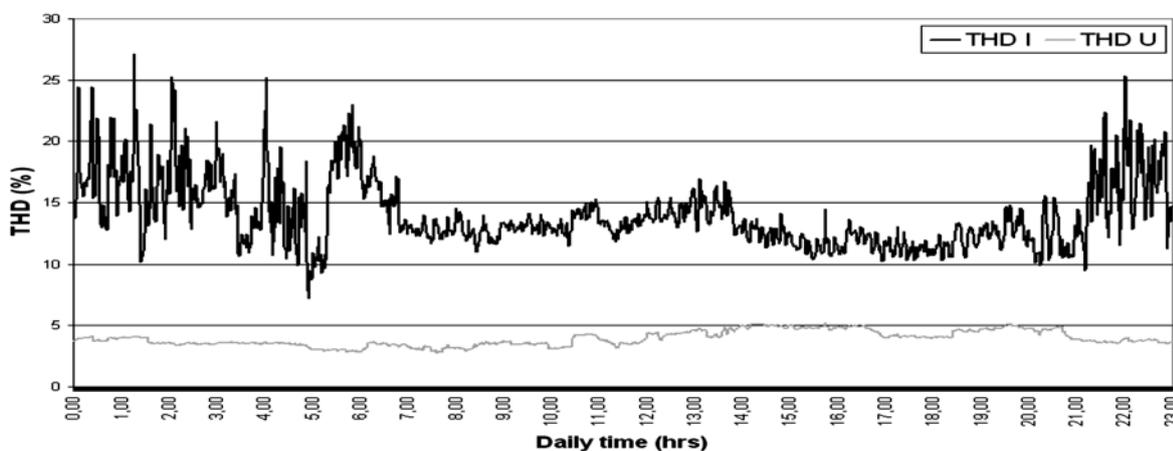
Figure 5 Period diagram THDU and THDI for non-linear load
