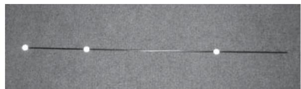
Figure 2. Wand calibration. Second calibration step – refinement of camera parameters. Single calibration wand used for 'wand dance'.
