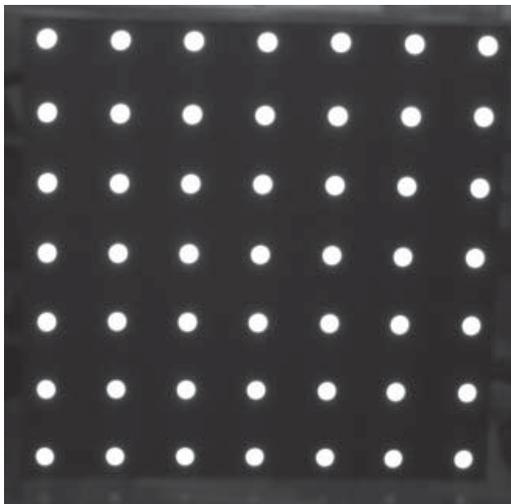
Figure 3. 2D plate calibration.  $7 \times 7$  co-planar circular calibration points. The diameter of the circles is 20mm and they are 150mm apart.
