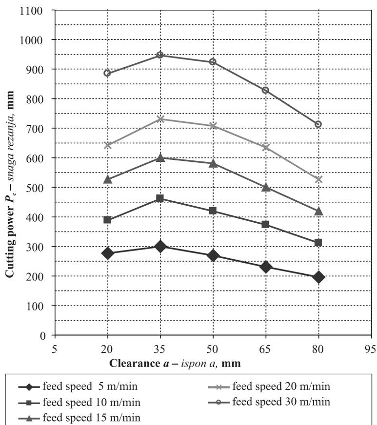
**Figure 2** The influence of the clearance of saw blade over the workpiece on the cutting power with individual feed speed for saw blade with carbide
