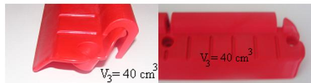
Figure 8. Uninjected products at a lowering switch point
