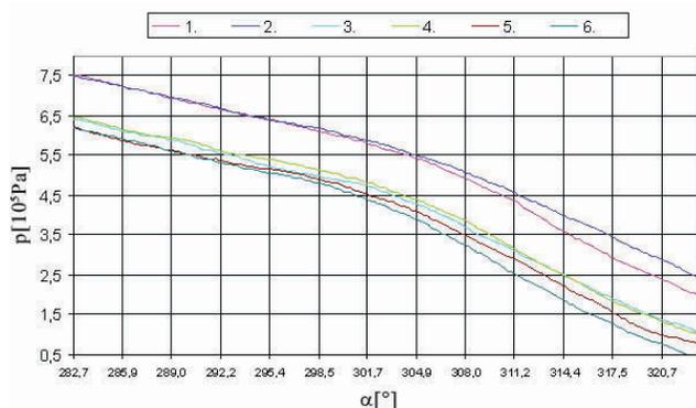
Figure 16 Cylinder pressure curve at exhaust valve opening segments on all cylinders at 100% load
