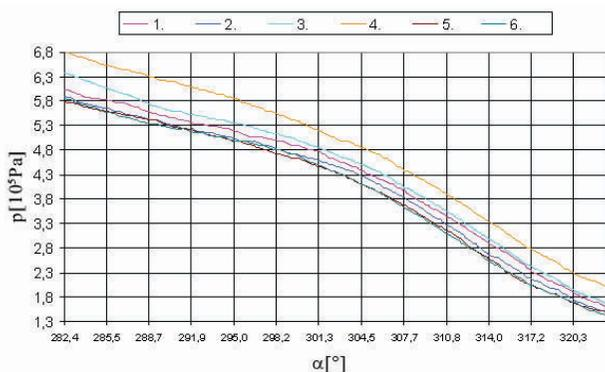
Figure 28 **Cylinder pressure curves at exhaust valve opening segments in all six cylinders at 75% load**
