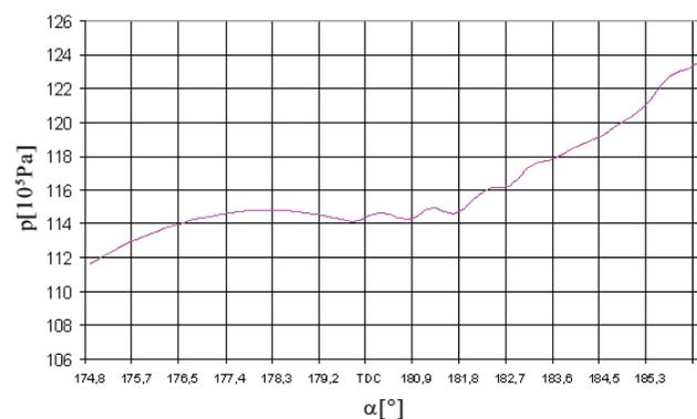
Figure 14 **Cylinder pressure curve segments in the fifth cylinder at 100% load**
