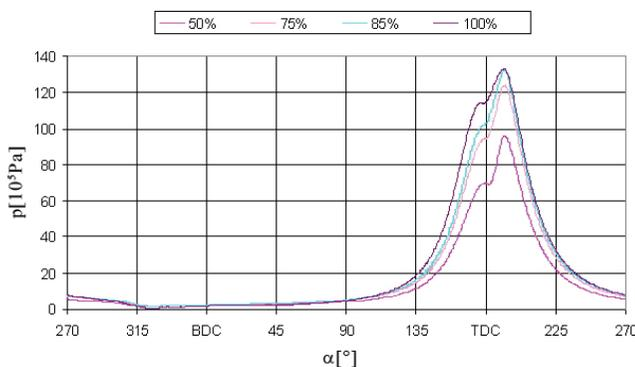
Figure 6 **Cylinder pressure in sixth cylinder at different loads**
