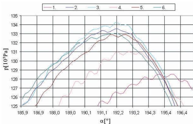
Figure 8 Cylinder pressure curves, combustion segments, in all cylinders at 100% load
