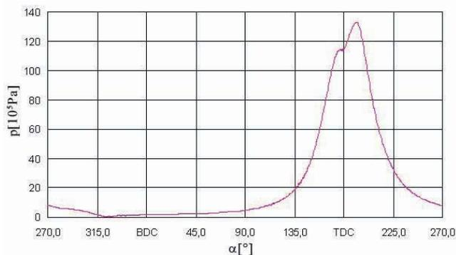
Figure 3 **Cylinder pressure in the sixth cylinder at 100% load**
