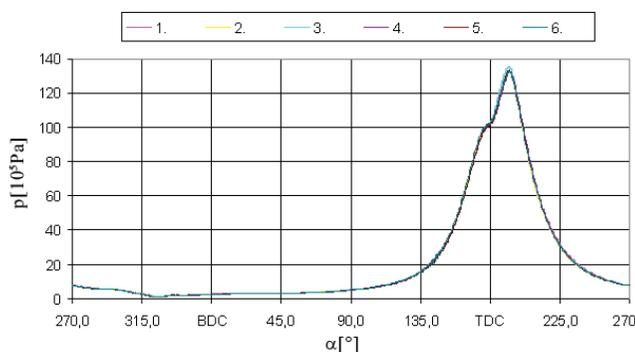
Figure 18 Cylinder pressure in all cylinders at 85% load
