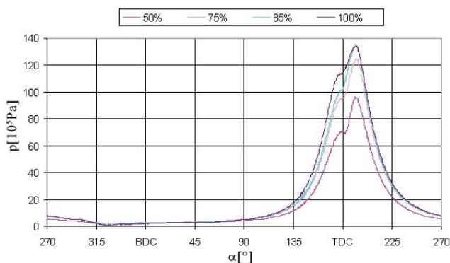
Figure 5 **Cylinder pressure in the third cylinder at different loads**
