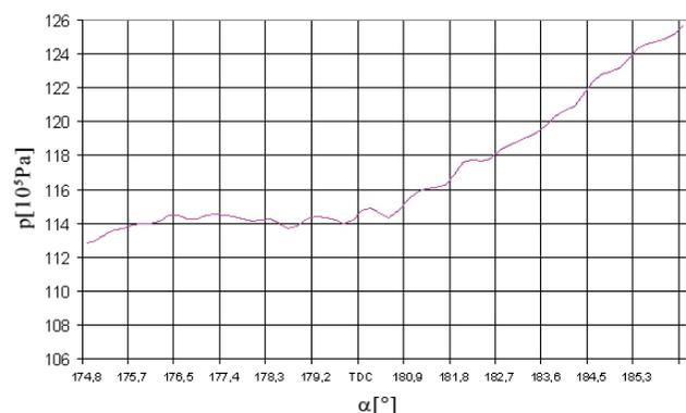
Figure 15 **Cylinder pressure curve segments in the sixth cylinder at 100% load**
