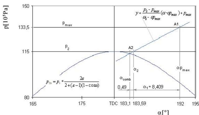
Figure 2 **Compression pressure curve in correlation with the crank angle and straight line construction at 100% load**
