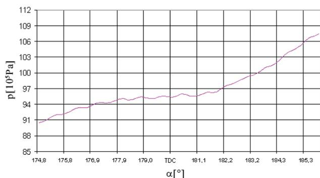
Figure 24 **Cylinder pressure curve segments in the third cylinder at 75% load**
