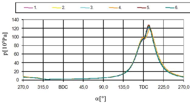
Figure 19 **Cylinder pressure in all cylinders at 75% load**
