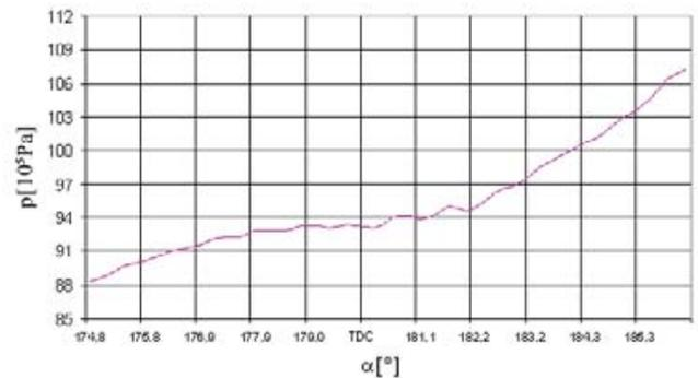
Figure 22 **Cylinder pressure curve segments in the first cylinder at 75% load**
