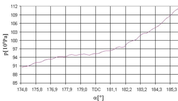
Figure 25 **Cylinder pressure curve segments in the fourth cylinder at 75% load**
