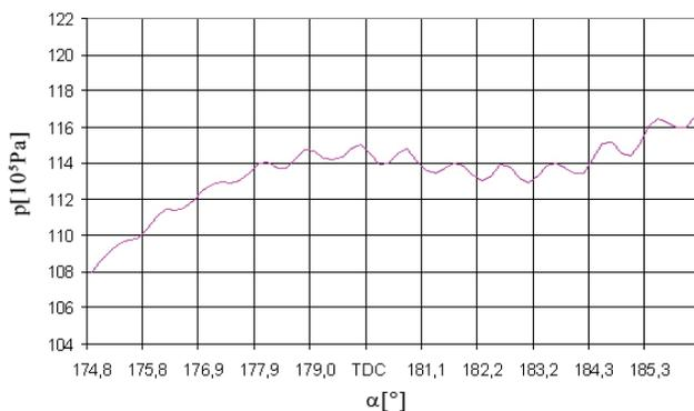
Figure 10 Cylinder pressure curve segments in the first cylinder at 100% load
