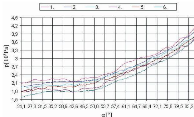
Figure 17 Cylinder pressure curve at scavenging port closing segments on all cylinders at 100% load
