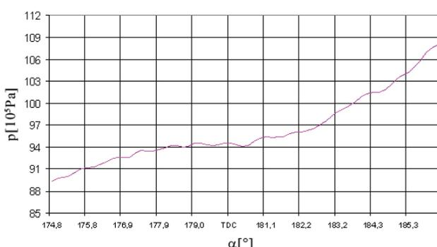
Figure 27 **Cylinder pressure curve segments in the sixth cylinder at 75% load**
