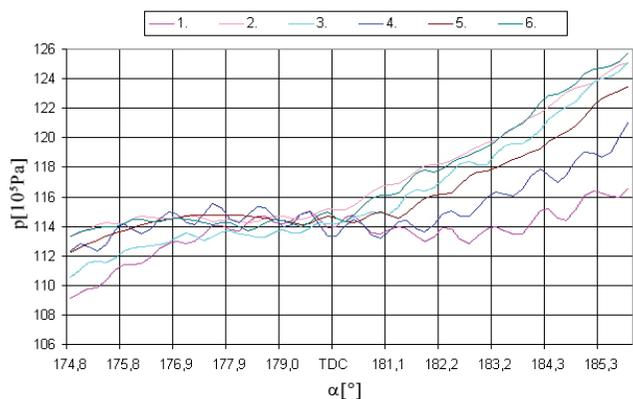
Figure 9 Cylinder pressure curves, injection segments, in all cylinders at 100% load
