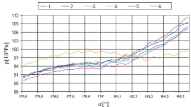
Figure 21 **Cylinder pressure curves, injection segments, in all cylinders at 75% load**
