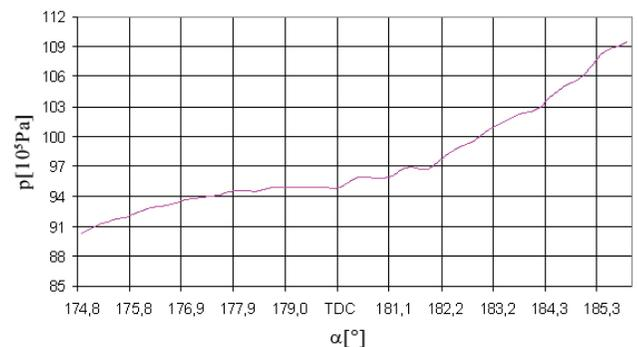
Figure 23 **Cylinder pressure curve segments in the second cylinder at 75% load**
