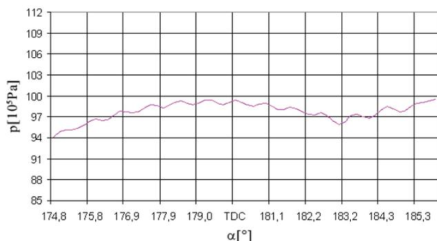
Figure 26 **Cylinder pressure curve segments in the fifth cylinder at 75% load**
