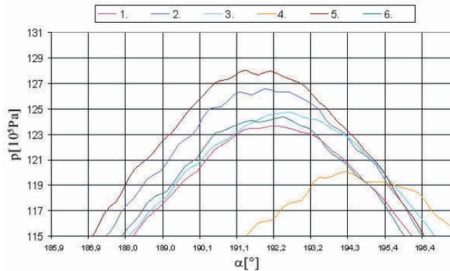
Figure 20 **Cylinder pressure curves, combustion segments, in all cylinders at 75% load**
