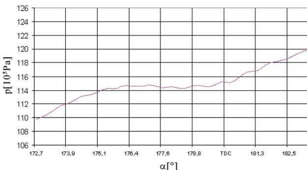
Figure 11 Cylinder pressure curve segments in the second cylinder at 100% load
