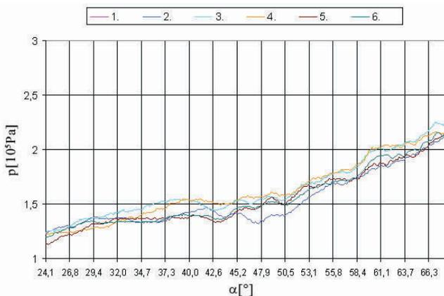
Figure 29 **Cylinder pressure curves at scavenging port closing segments in all six cylinders at 75% load**
