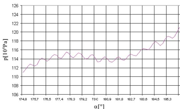
Figure 13 **Cylinder pressure curve segments in the fourth cylinder at 100% load**
