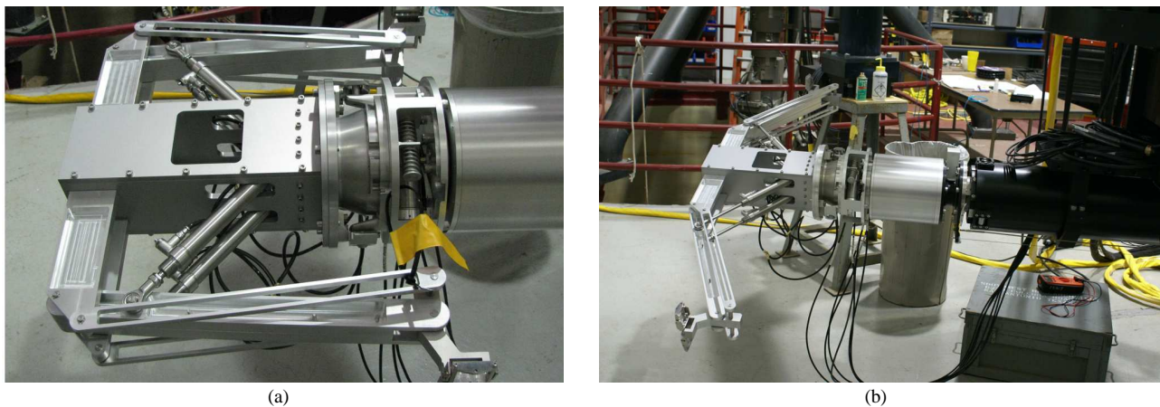
Fig. 8. Two working positions of nozzle inspection tool
