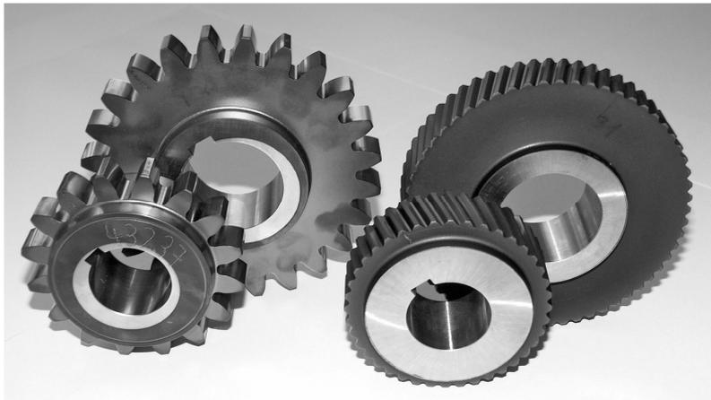
Fig. 13: Geometry of standard C type gears and lowloss gears
