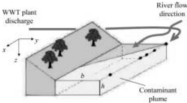
Fig. 1 – Schematic representation of a riverine pathway contamination with a pollutant release from a WWTP (small size release point located in the middle of the river; adapted from Whelan & McDonald<sup>24</sup>)
