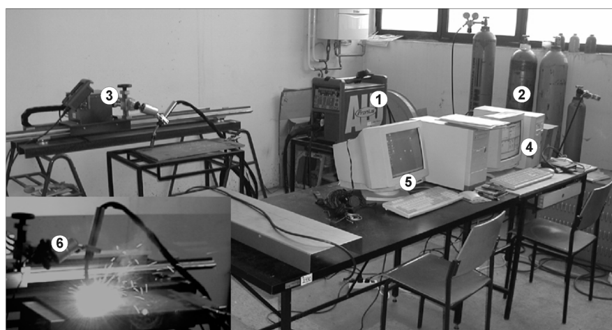
Figure 2. Laboratory system for monitoring, acquisition and processing of main welding parameters [18]
