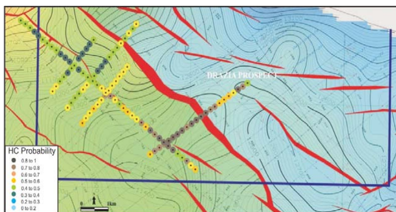
Fig. 9. Top Alam El Bueib depth map & probability of success based on acoustic spectroscopy
